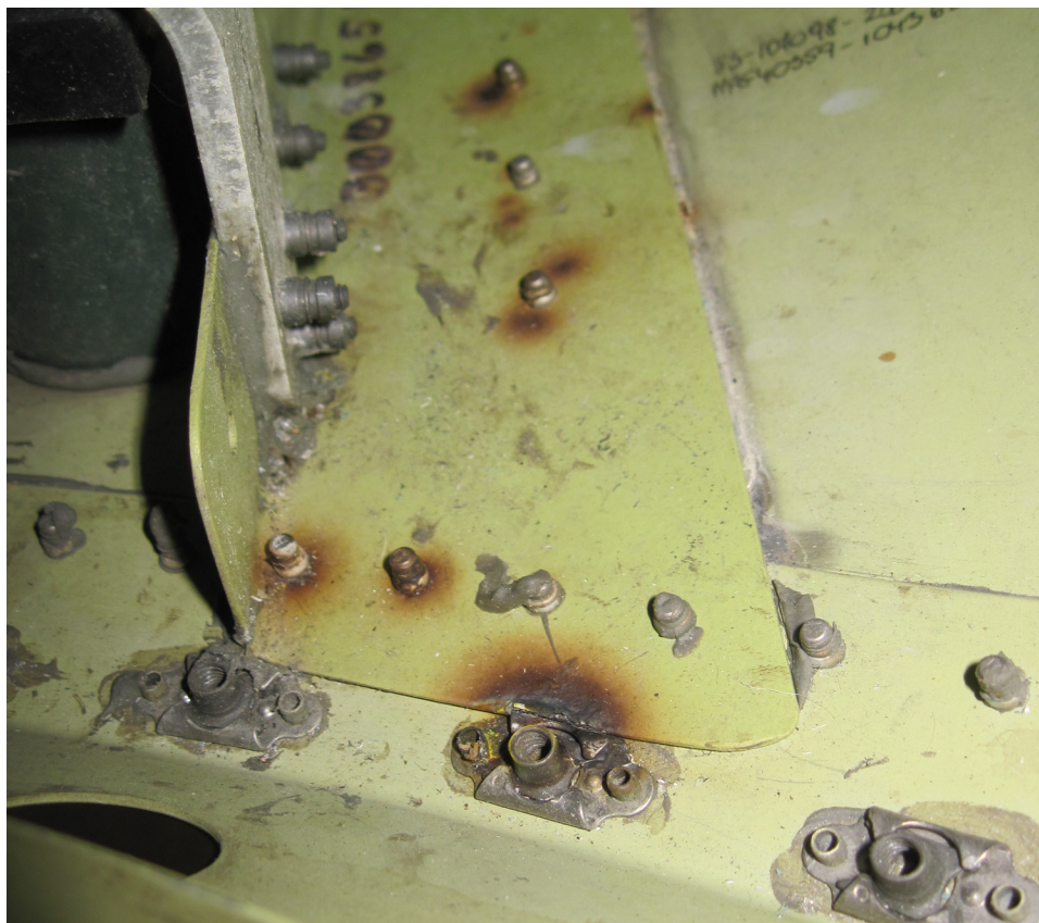
Figure 4. Internal Electrical Damage
