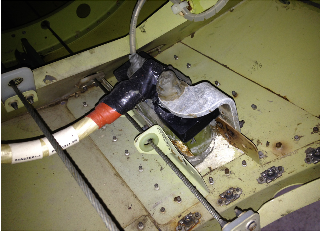
Figure 5. Internal Electrical Damage
