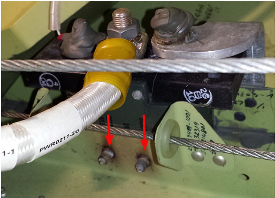
Figure 6. Internal Electrical Damage
