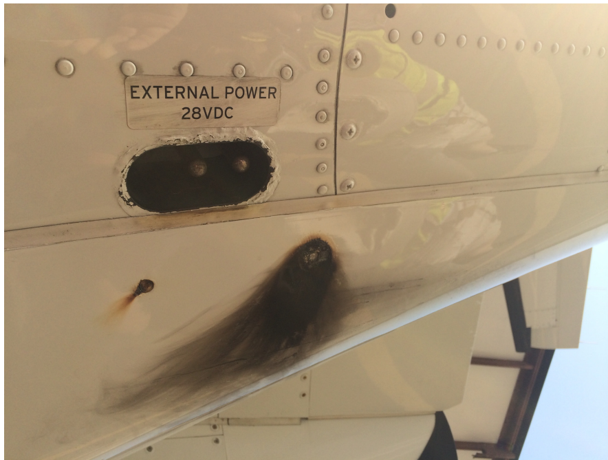
Figure 3. External Electrical Damage
